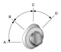
Using a tool to force the ignition control knob from its cylinder could damage it.
